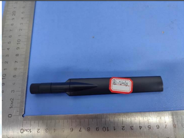
Antenna 9: 3.07dBi Dipole Antenna(AD-514AX)
