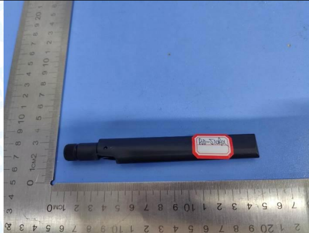
Antenna 8: 2.35dBi Dipole Antenna(AD-512AX)
