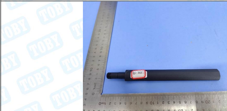
Antenna 3: 3.14dBi Dipole Antenna(AD-302N)
