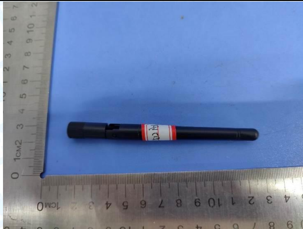
Antenna 9: 3.07dBi Dipole Antenna(AD-514AX)
