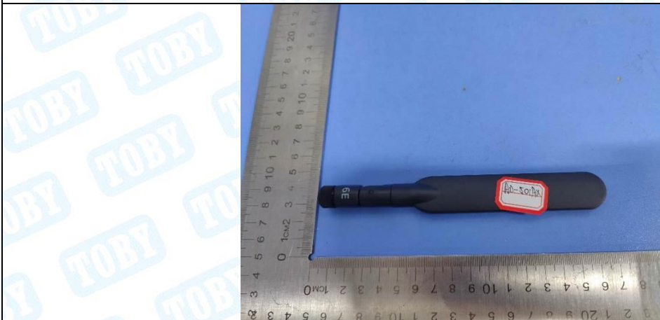
Antenna 6: 3.7dBi Dipole Antenna(AD-501AX)
