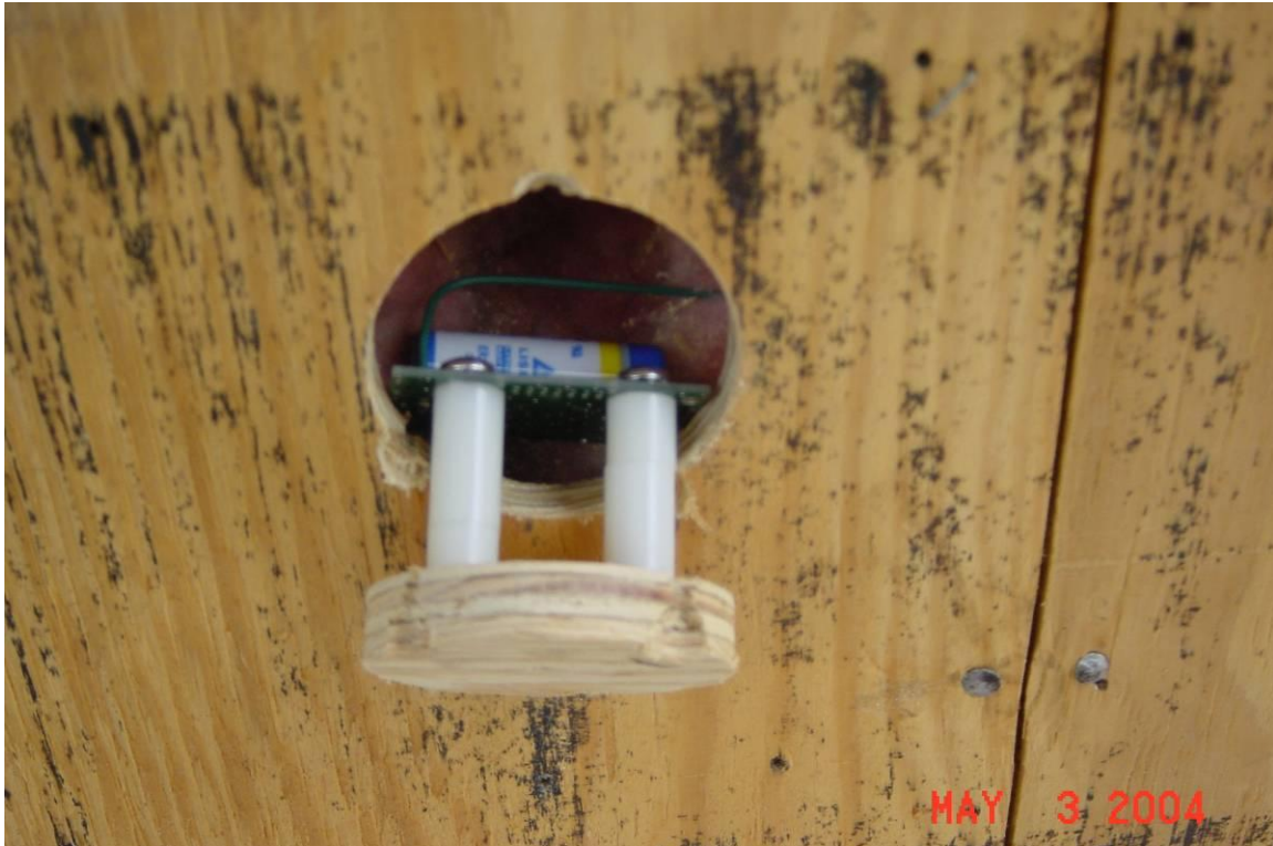
Figure 3 - Close up of Sensor Prior to Mounting from Exterior Side of Sheathing
