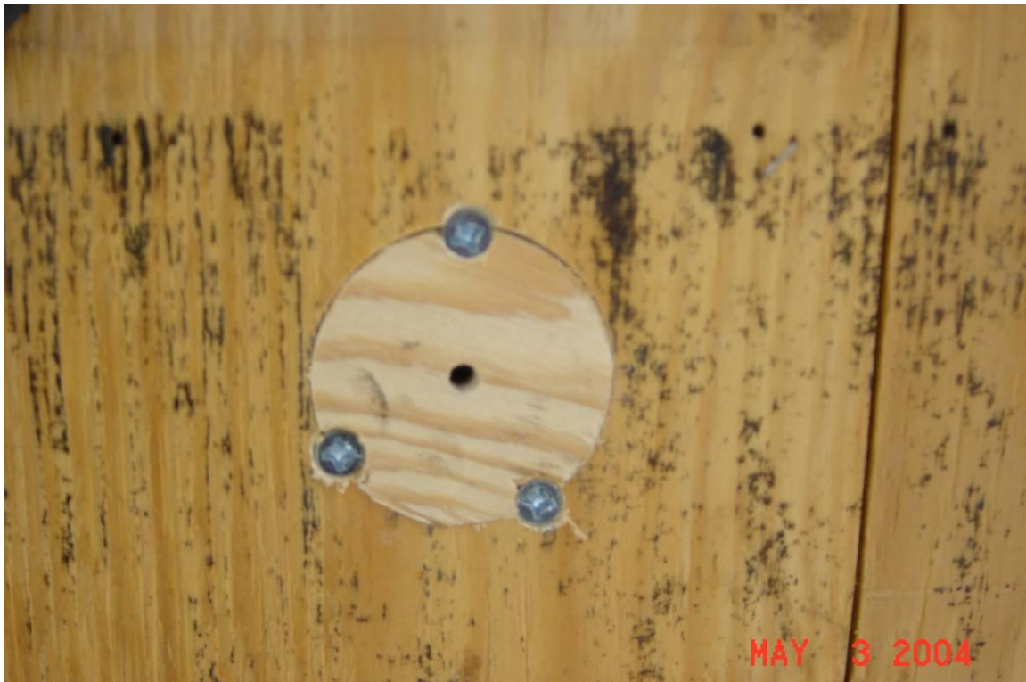
Figure 4 - Close up of Sensor Mounted from Exterior Side of Sheathing
