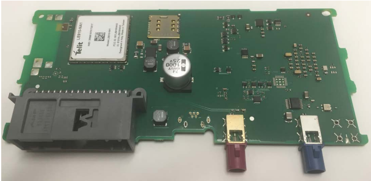
Figure 1.- FTM mounted PCB top view
