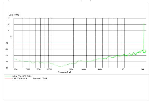
A.5.3.2 RADIATED SPURIOUS EMISSIONS-Channel 661: 30MHz – 2GHz NOTE: peak above the limit line is the Carrier frequency @ ch-661
