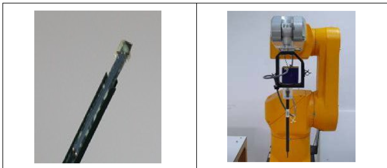
EX3DV4 E-field Probe
