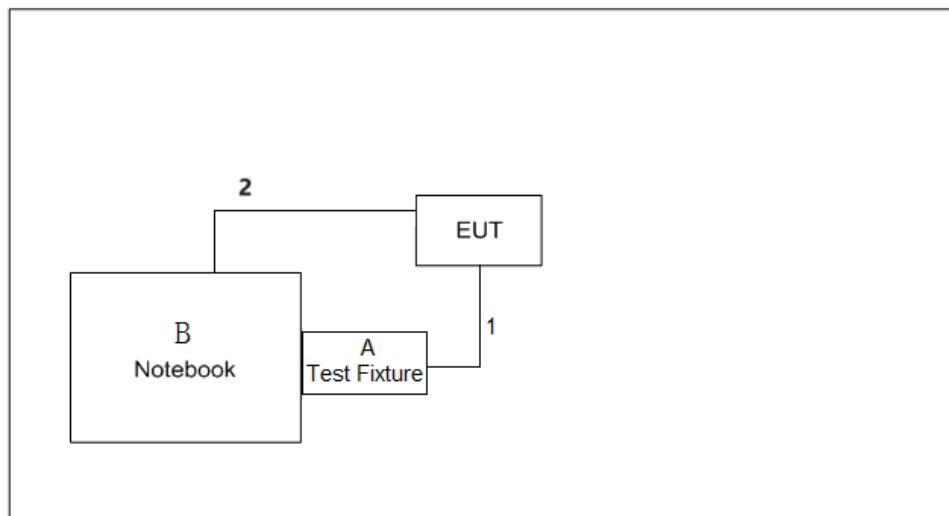
Radiated emissions test – Above 18GHz
