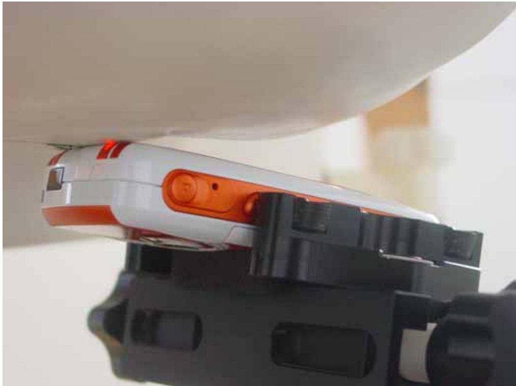
Picture B3: Right Hand Tilt 15° Position with Bluetooth transmitter ON
