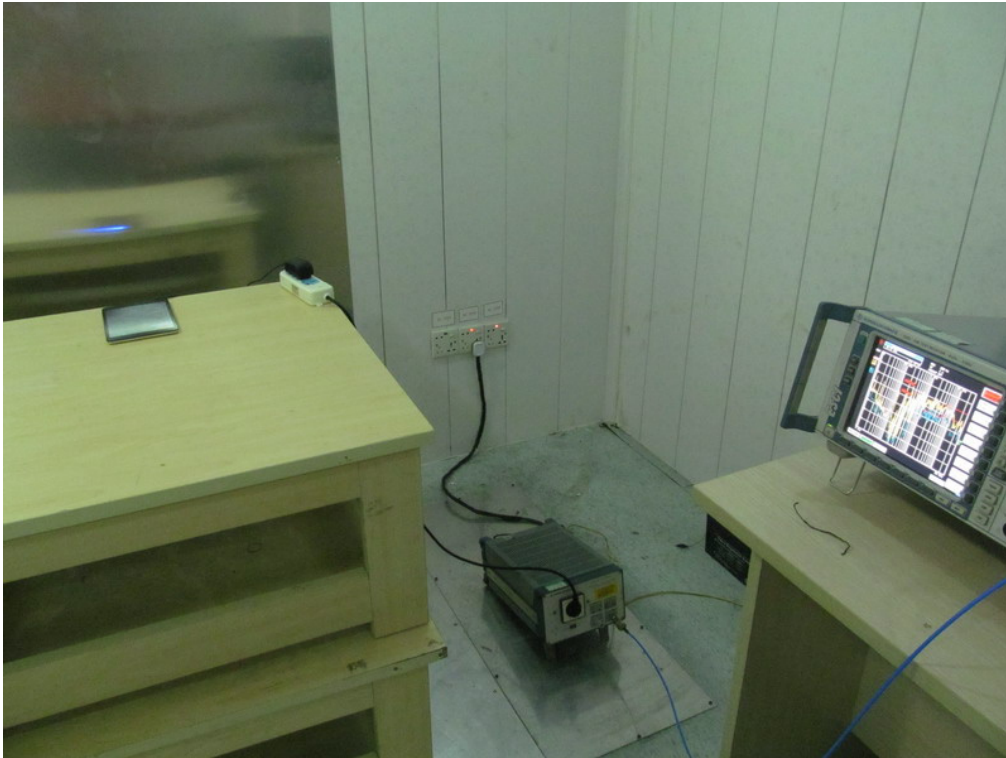
FCC RADIATED EMISSION TEST SETUP
