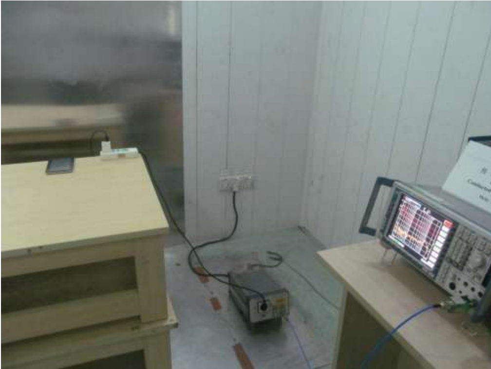
FCC RADIATED EMISSION TEST SETUP
