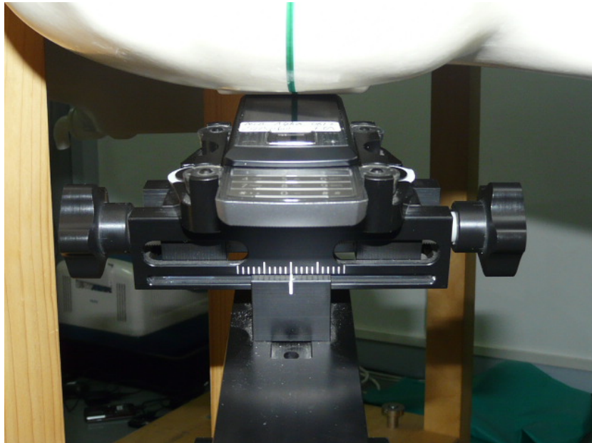
Picture 4: Head SAR tilt position 1
