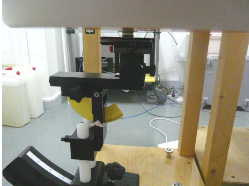
Picture 6: Body SAR Back to the phantom
