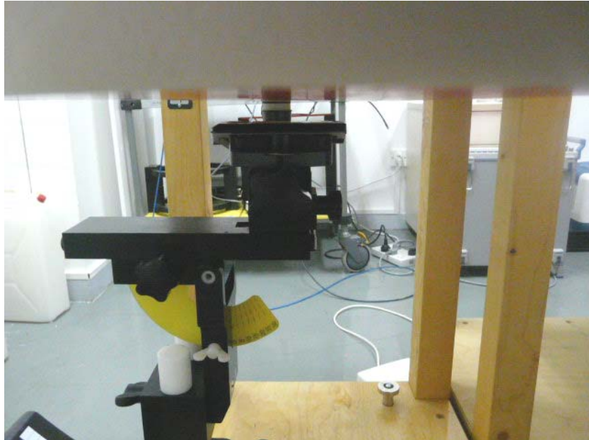
Picture 7: Body SAR Front to the phantom
