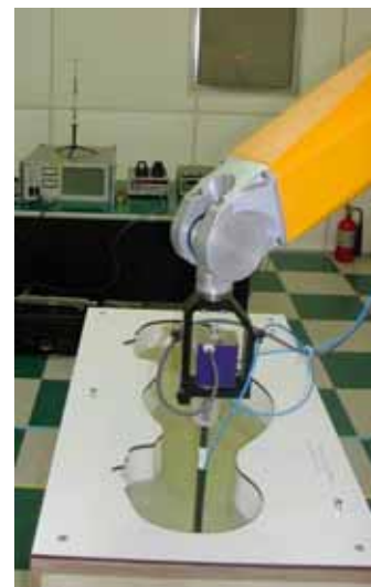
Figure 4. Photograph of the probe and the Phantom
