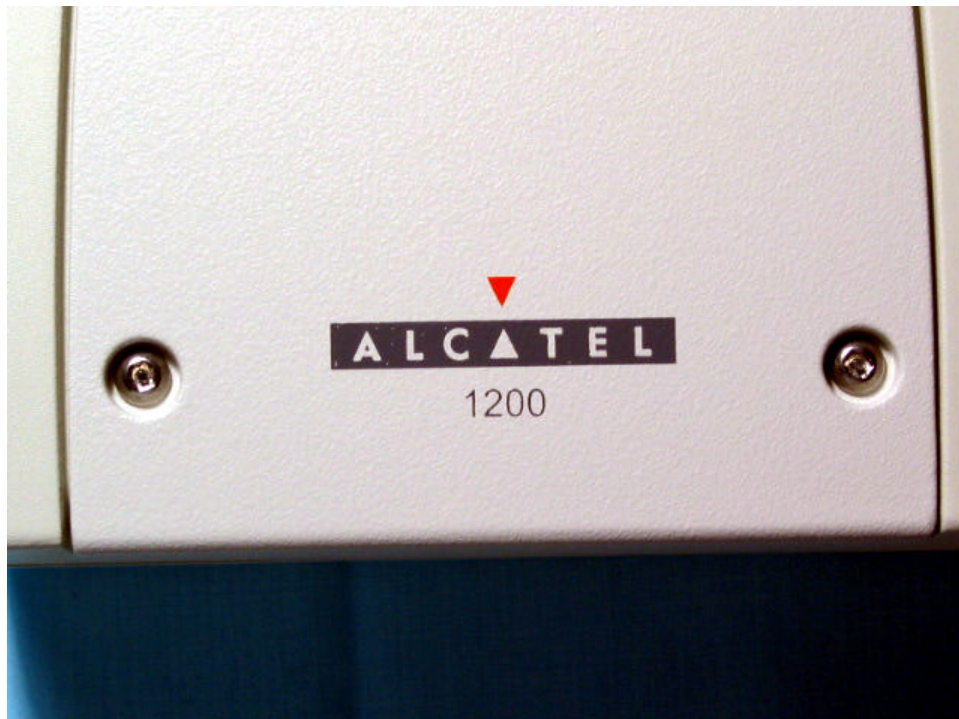
Alcatel Access Point, Models 1200B and 1200B INT Security Screw detail
