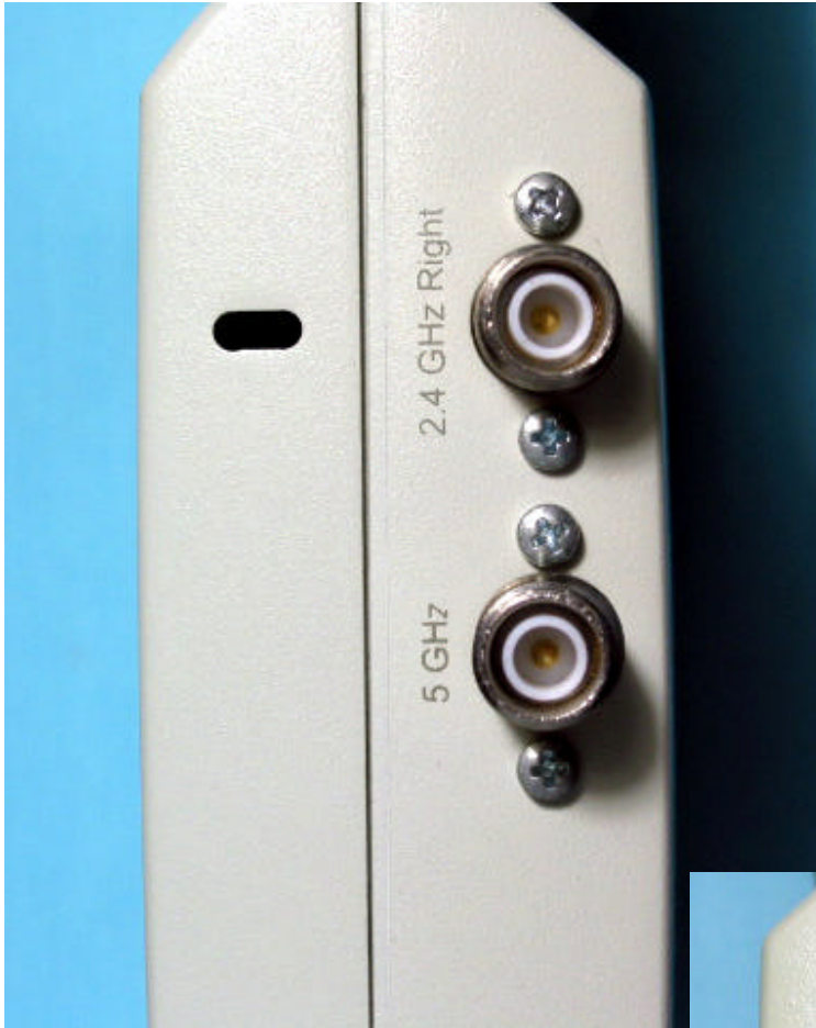
Alcatel Access Point, Connector Detail Model 1200
