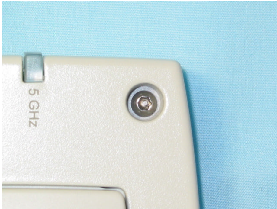
Alcatel Access Point, Models 1200 and 1200 INT Security Screw detail
