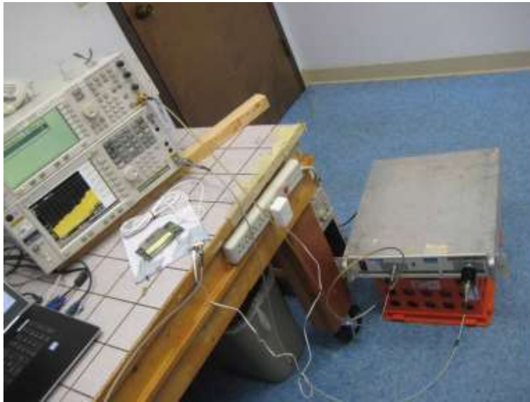
Section 7.2-7.3 UL Test Setup, Max Power Input Signal
