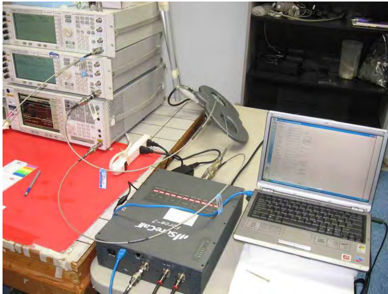
Section 7.9.2 Variable Gain Test Setup
