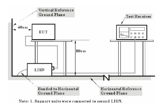
The setup of EUT is according with per MP-5: 1986 measurement procedure. Specification used was with
