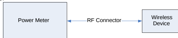
Figure 10-1 Power Measurement Setup
