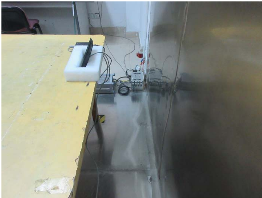
Conducted Emissions Test Setup Side View
