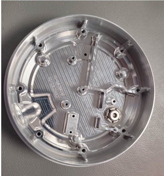
Yahsat T-TAC Maritime Antenna Step 1 – Mounting of TNC Connector
