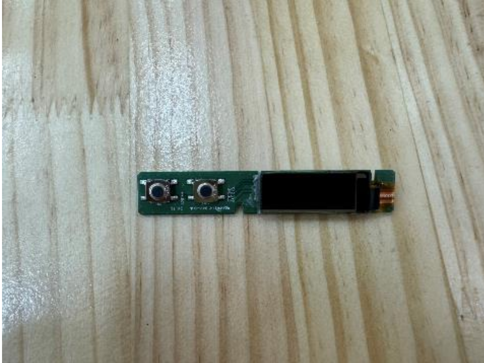
Rear View of OLED Board_EXPD 4343N1, EXPD 3643N1
