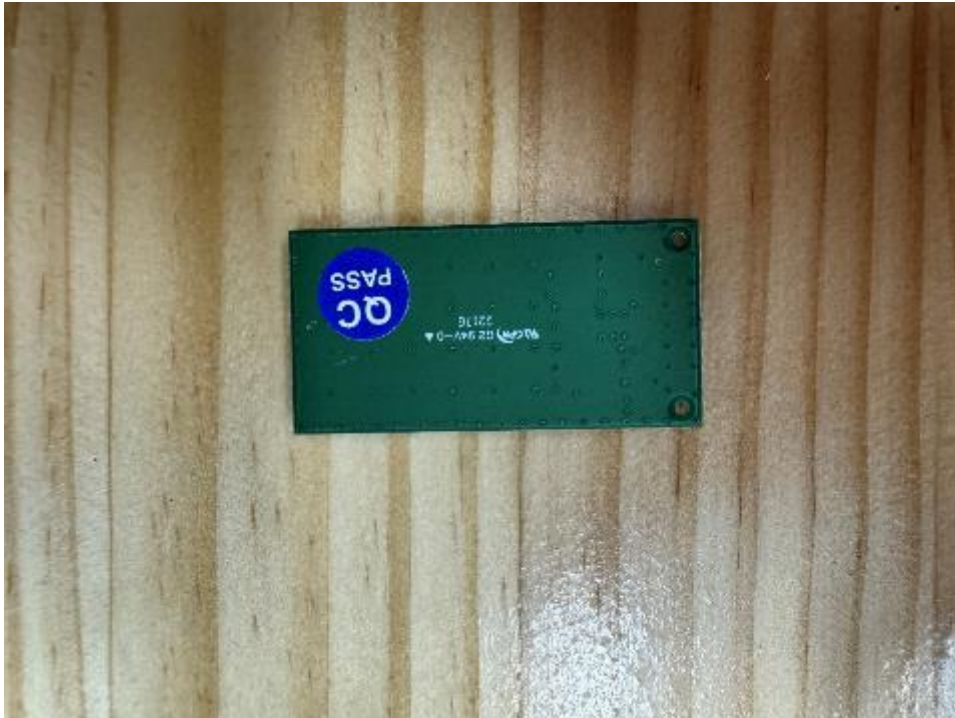
Rear View of WiFi module Board_EXPD 4343N1, EXPD 3643N1
