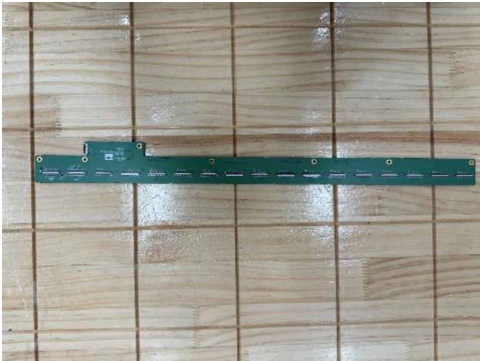
Rear View of ROIC Board_EXPD 4343N1
