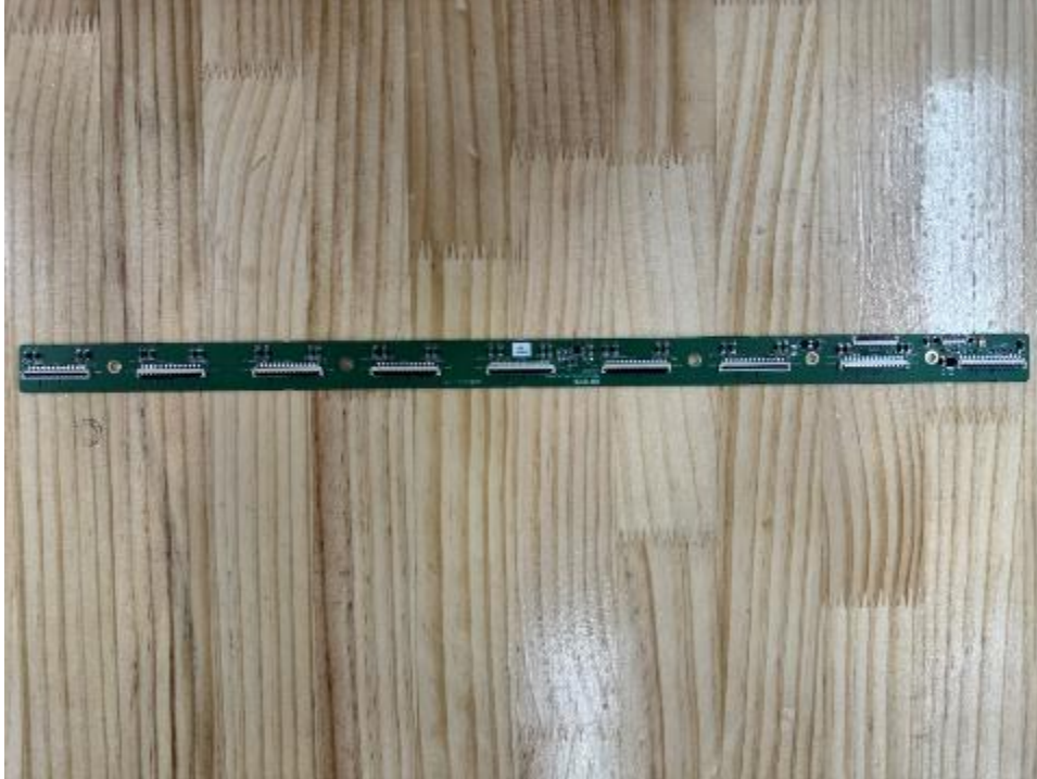
Rear View of Gate Board_EXPD 4343N1, EXPD 3643N1
