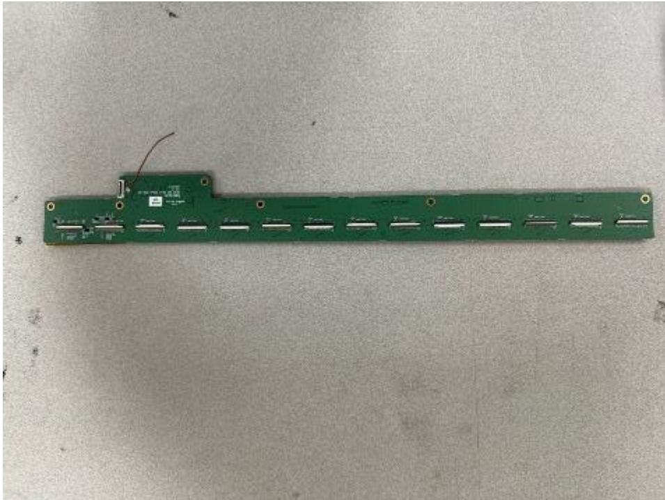
Rear View of ROIC Board_EXPD 3643N1
