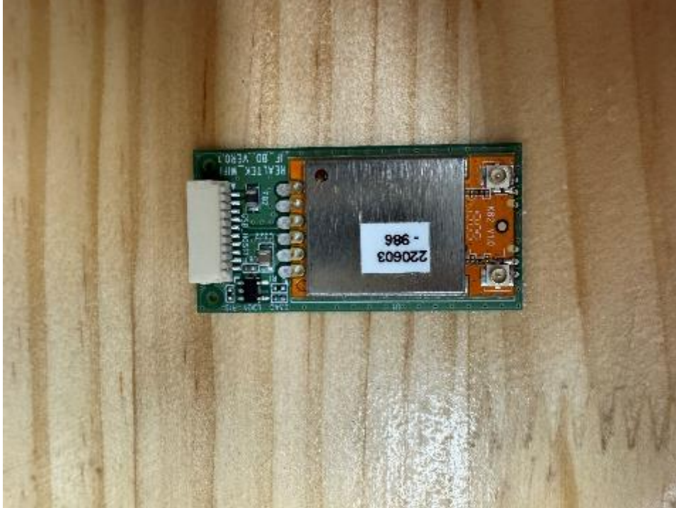
Rear View of WiFi module Board_EXPD 4343N1, EXPD 3643N1
