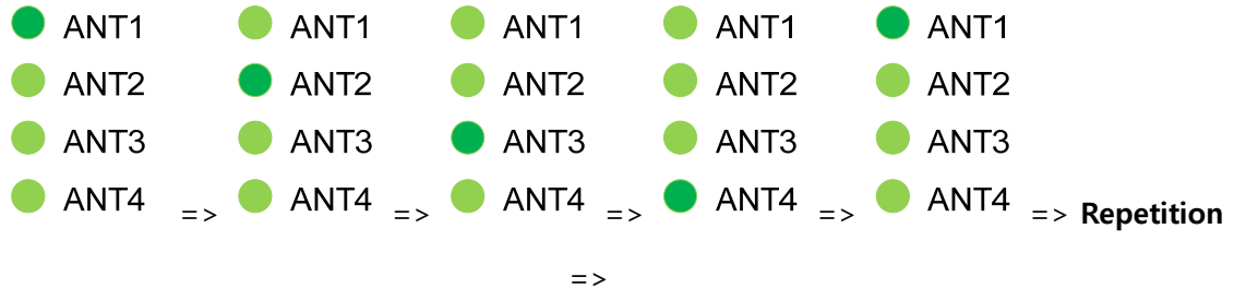
<Fig. 12> LED for indicating antenna channel
