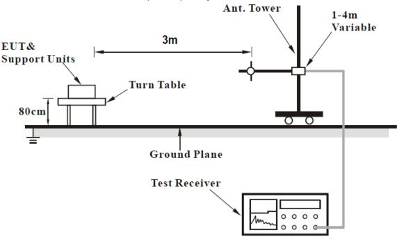
(B) Radiated Emission Test Set-Up, Frequency above 1000 MHz
