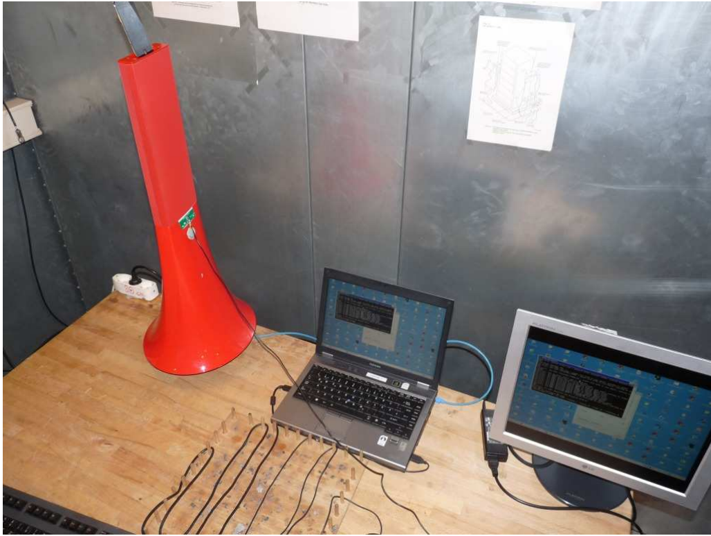
Photo 4: Test setup for conducted measurements, AC Mains
