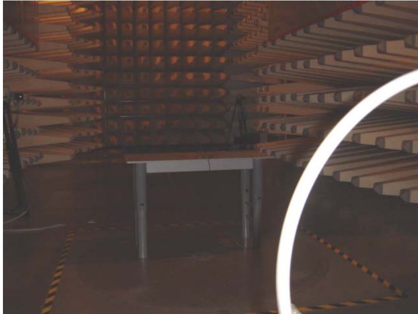
Set-up for Radiation Emission (Transceiver)
