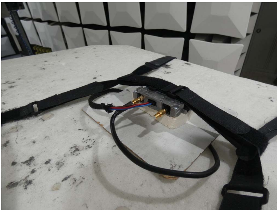
Photo 2: Test setup used for the test case “Radiated spurious emissions” FCC § 20.21 in the range 1000 MHz -20 GHz, detailed view.
