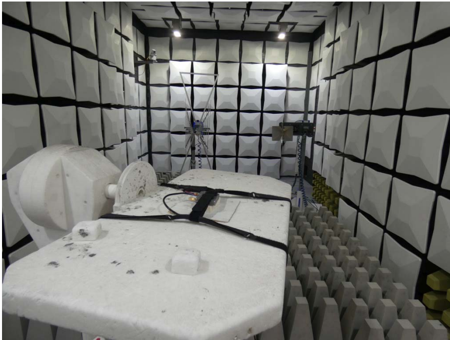
Photo 1: Test setup used for the test case “Radiated spurious emissions” FCC § 20.21 in the range 1000 MHz -20 GHz.
