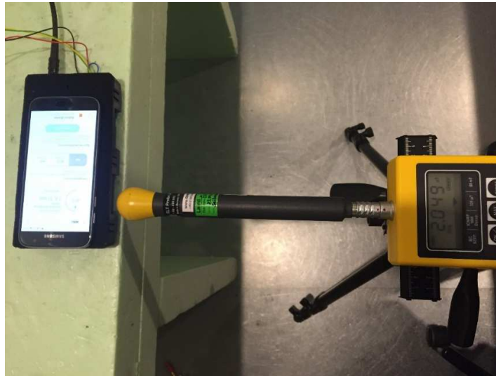
Worst case position H-field probe (right coil, pos C, 2.5 cm)
