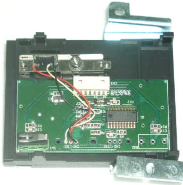
Solder side view of Card Reader board
