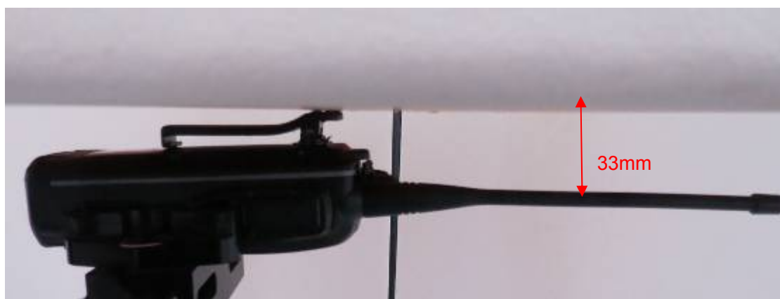
Picture 6: Body-worn, the front of the EUT towards ground, Belt clip directed tightly to touch the bottom of the flat phantom, the distance from the EUT Antenna to the bottom of the Phantom is 33mm
