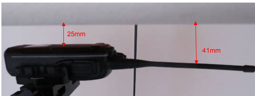
Picture 5: Face-held, the front of the EUT towards phantom, the distance from the EUT Antenna to the bottom of the Phantom is 41mm
