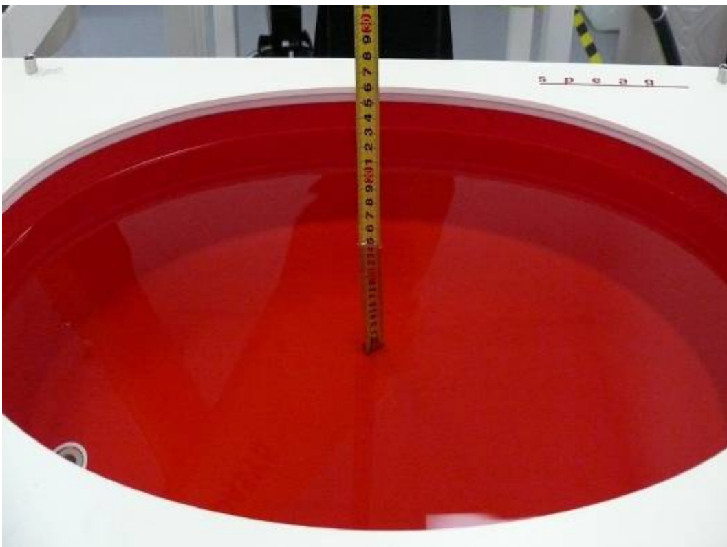
Picture 3: Liquid depth in the Flat Phantom (300MHz, 15.4cm depth)
