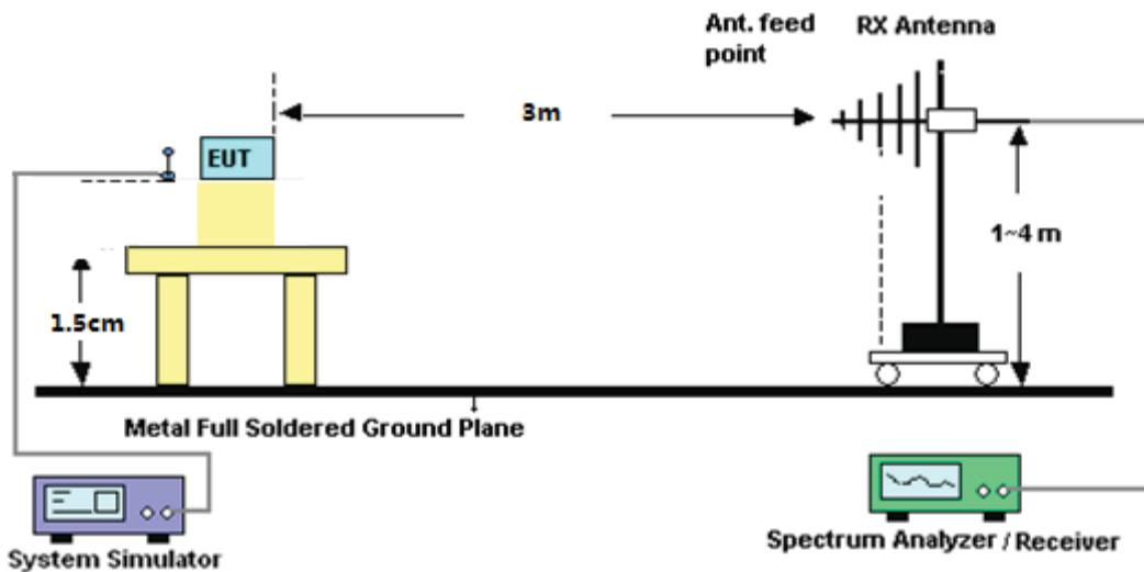
For radiated test from above 1GHz
