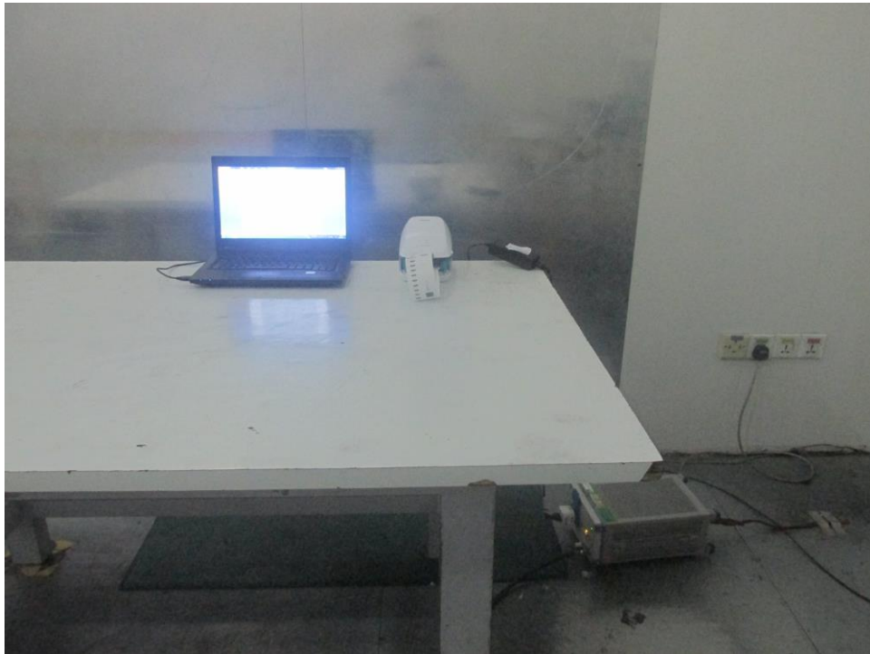
Photograph 2: Setup for Conducted emissions on AC Mains
