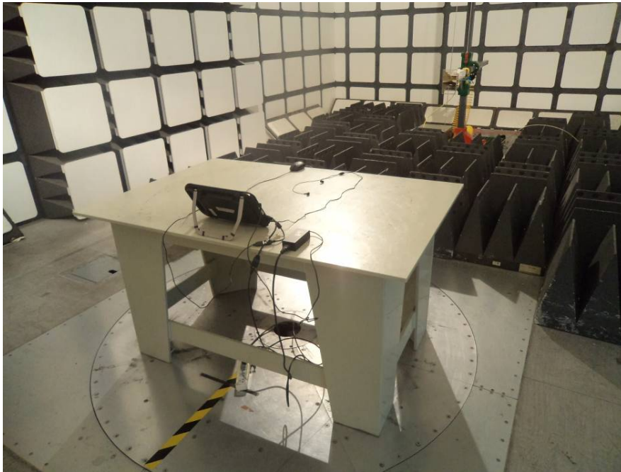
Above 1 GHz: Radiated Emissions – Rear View
