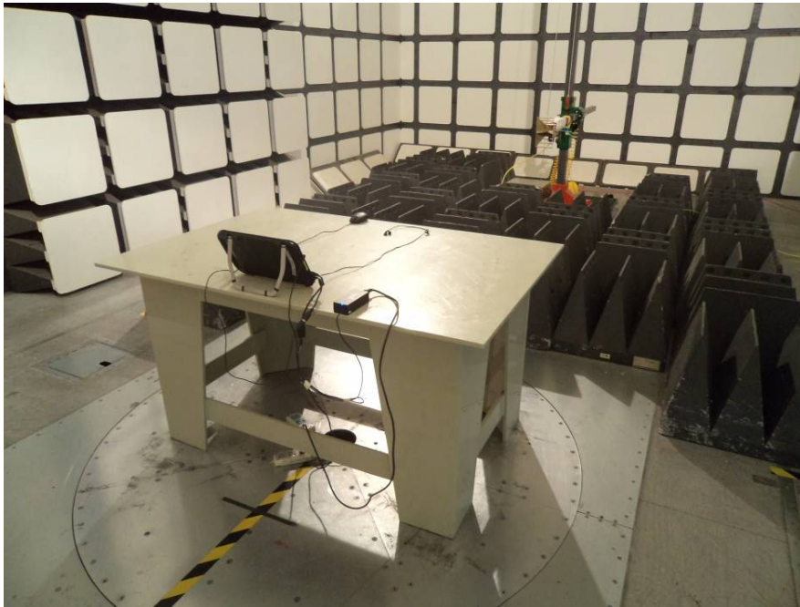
Above 1 GHz: Radiated Emissions – Rear View
