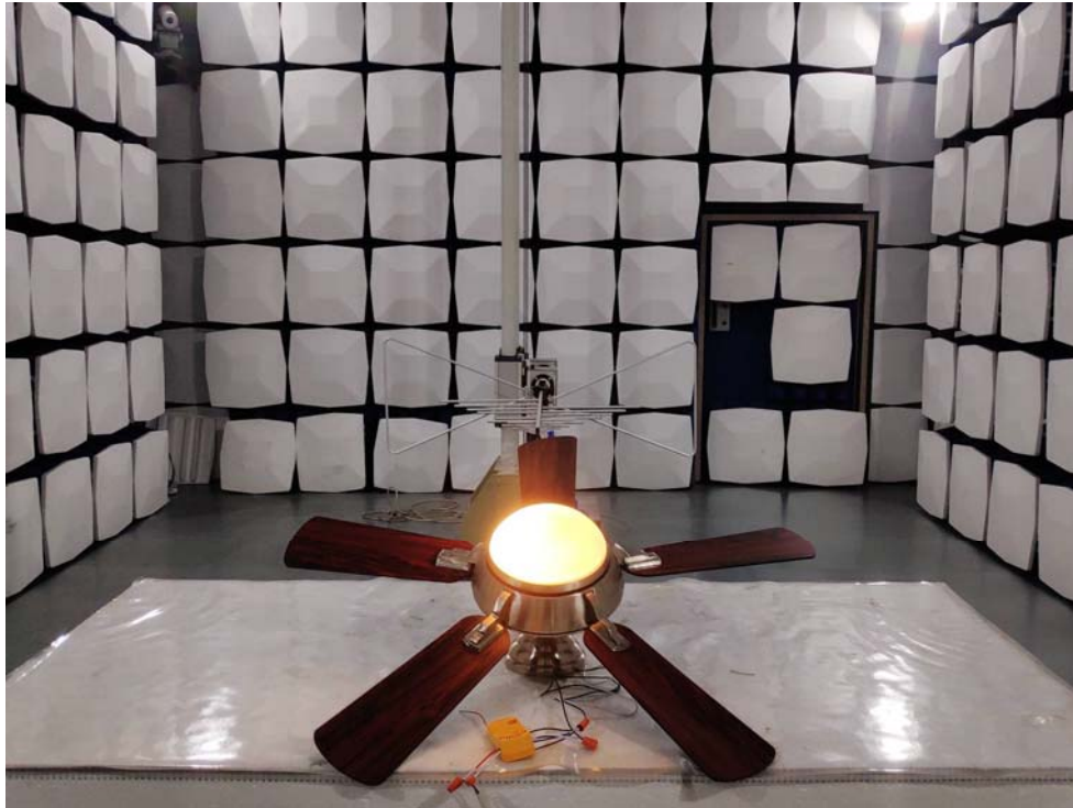
Radiated Emission Test Setup:
