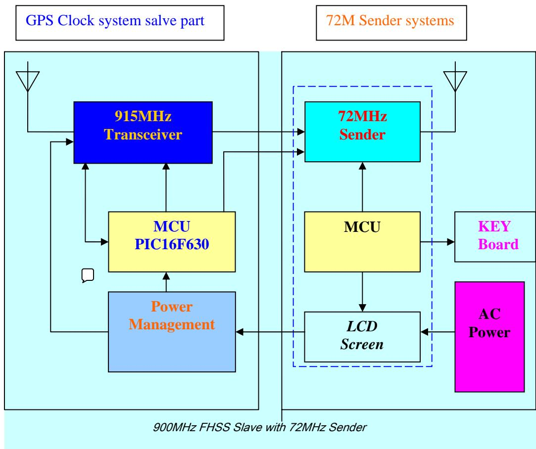
72MHz transmitting system and WGPS system are individual. WGPS HOST forward GPS time signal to WGPS SLAVE at WGPS system. Then WGPS SLAVE send time signal to 72 MHz transmitting system via RX-232 interface. 72MHz transmitting system had gotten FCC certification. (FCC ID: PZ3-FM72). The communication mode and socket is RS-232 at this system. But it is not standard RS -232 interface, not directly connect with PC.
