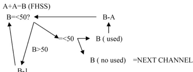
**b) Receiver starts to hop synchronically when receiving synchronic data. If it does not receive the data, it will be waiting in the random channel. The transmitter sends the channel information of next hopping frequency when transmitting while the receiver will send back ACK when receiving the signal and move to next channel defined by transmitter.**
