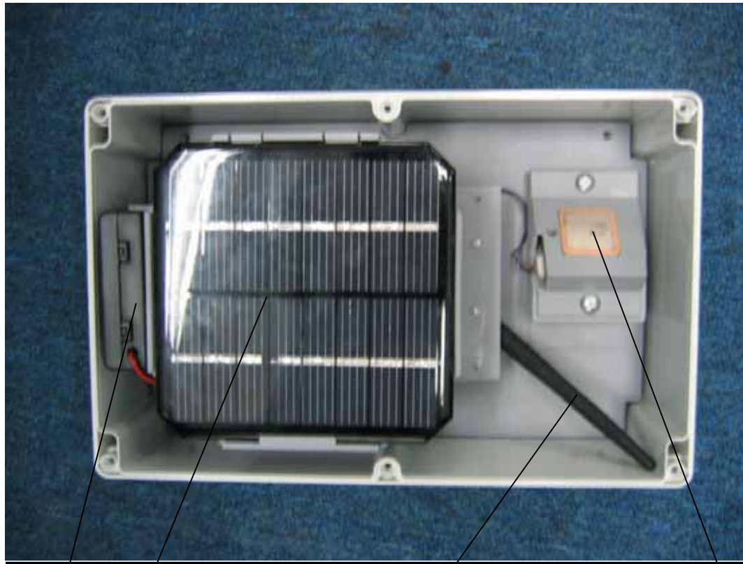
Solar panel NH rechargeable battery ATTENNA GPS
