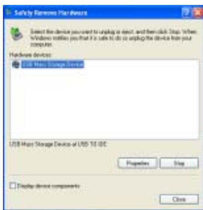
4. When the “Stop a Hardware Device” window appears, confirm the “USB Mass Storage Device” item and then press the [OK] button.
