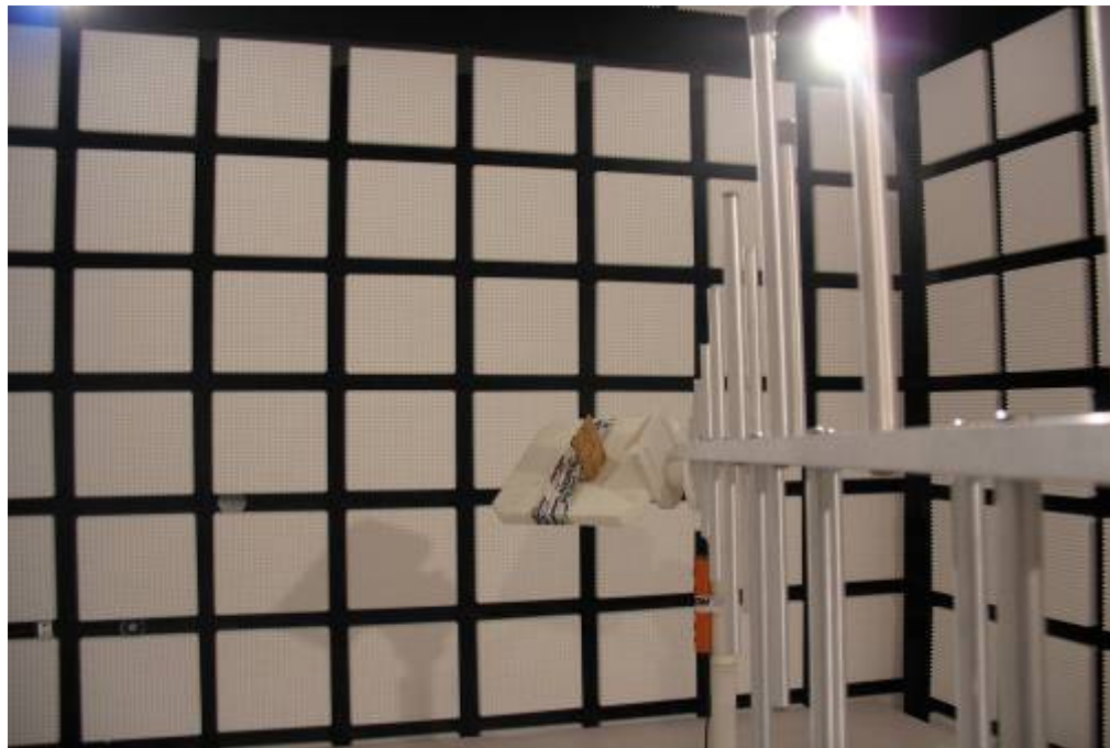
Photo 6: Position for max. E.I.R.P. (GFSK) DUT 40° / Azimuth 130°
