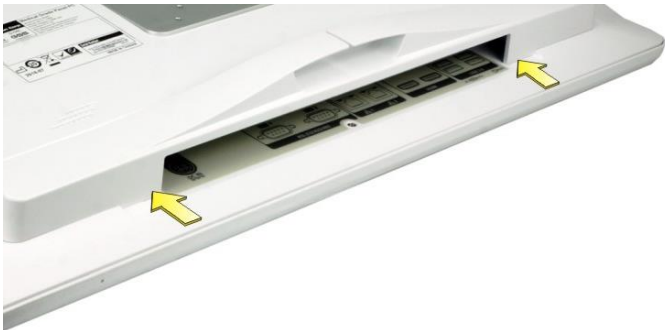
Figure 3-12: Cable Cover Removal
