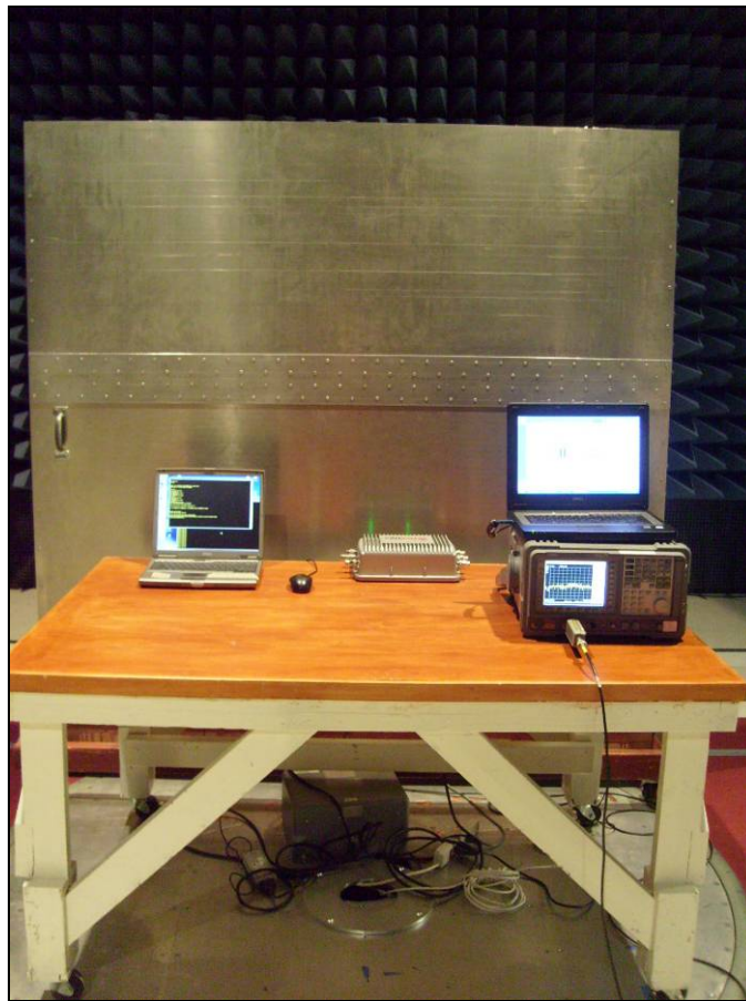
Photograph 7. Conducted Emissions, Test Setup
