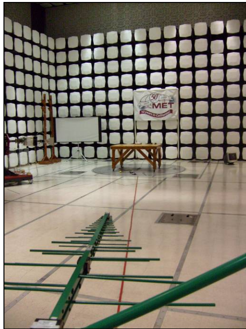
Photograph 5 Radiated Emission Test Setup 30 MHz – 1 GHz
