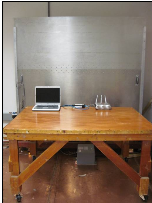
Photograph 3. Conducted Emissions, Test Setup 1
