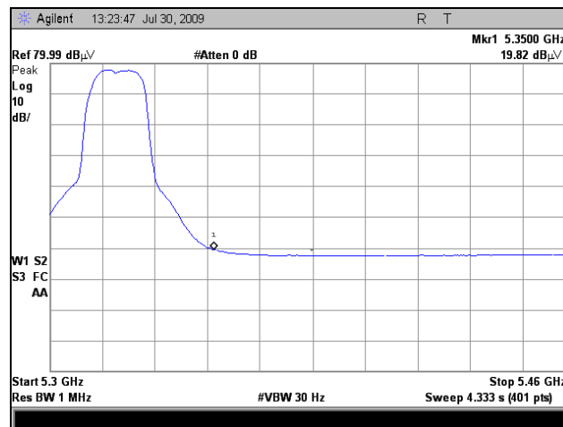
Plot 223. Restricted Band, 802.11n 20MHz, 5350 Average, 19 dBi Panel
