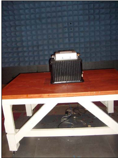
Photograph 2. Radiated Emission Spurious Test Setup
