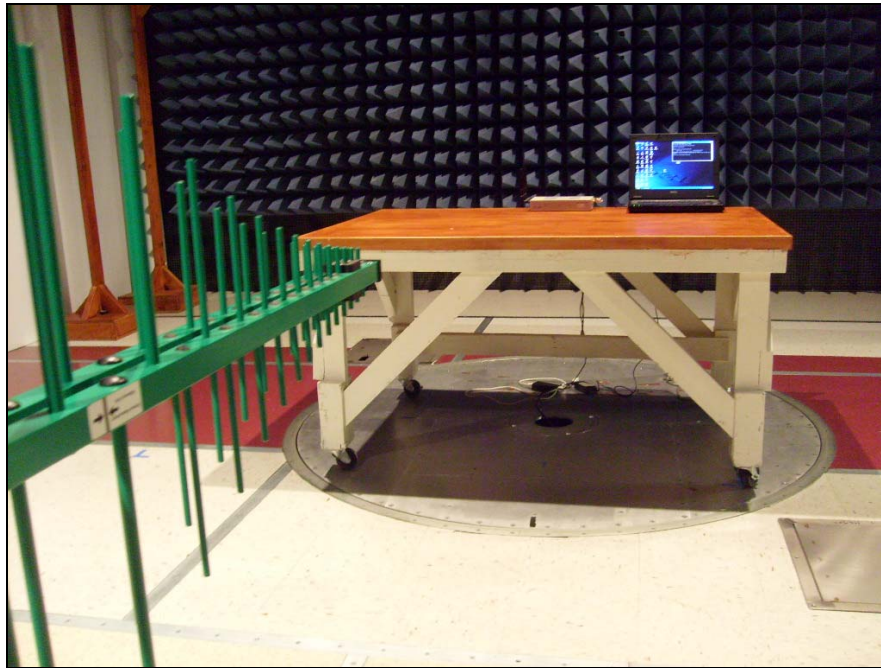
Photograph 3 Radiated Emission Test Setup 30 MHz – 1 GHz
