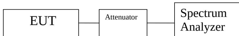
Figure 4. Peak Power Spectral Density Test Setup
