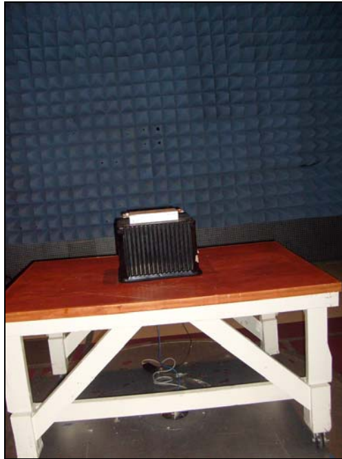
Photograph 2. Radiated Emission Spurious Test Setup, 1
