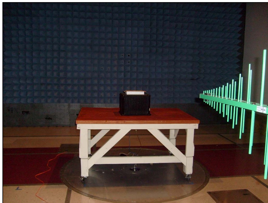
Photograph 3. Radiated Emission Spurious Test Setup, 2
