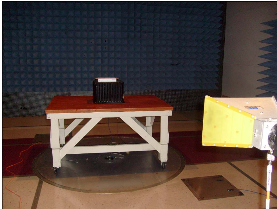
Photograph 4. Radiated Emission Spurious Test Setup, 3
