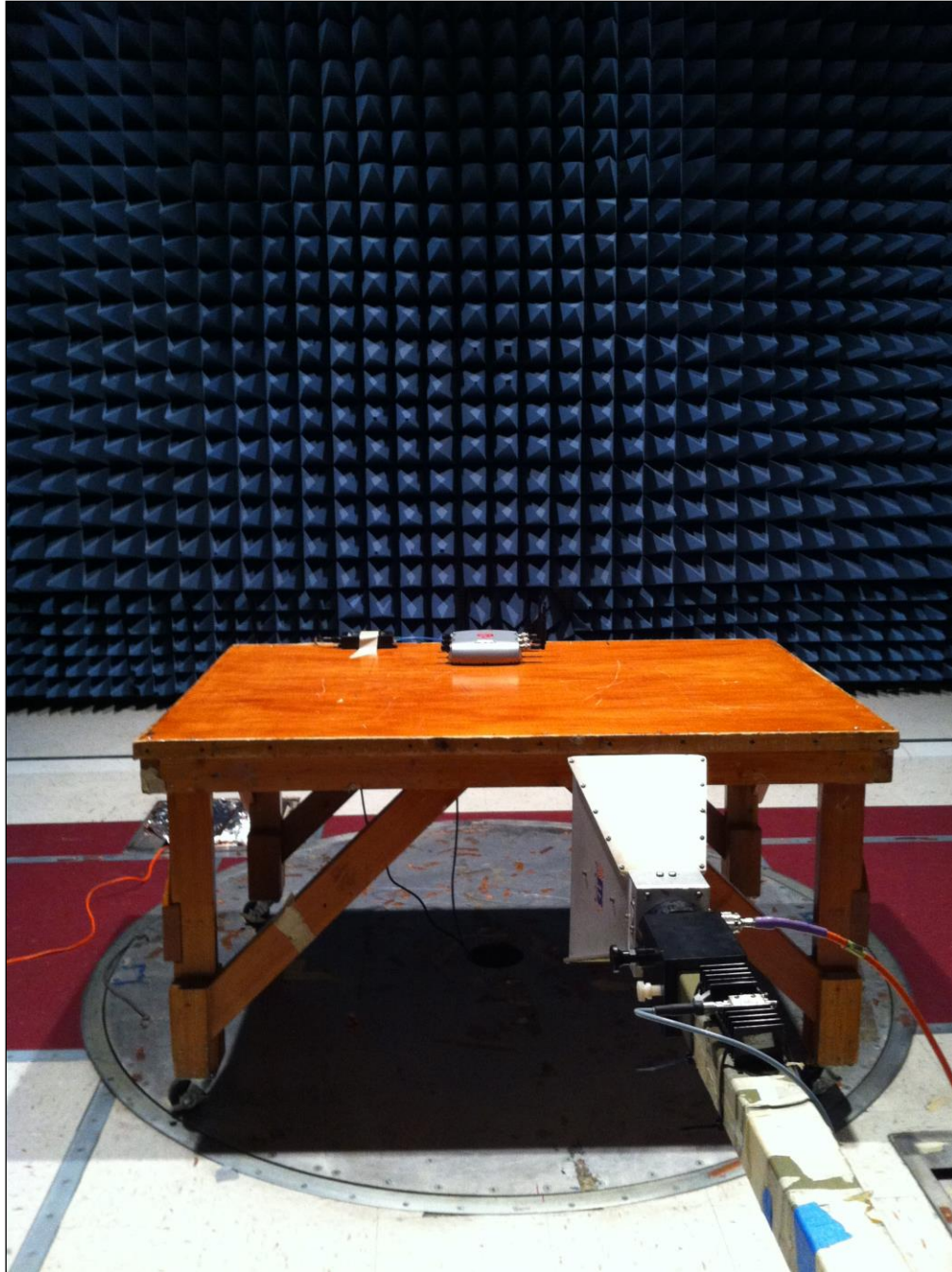
Photograph 8. Radiated Spurs, Test Setup, 5 dBi Omni, 1 GHz – 18 GHz
