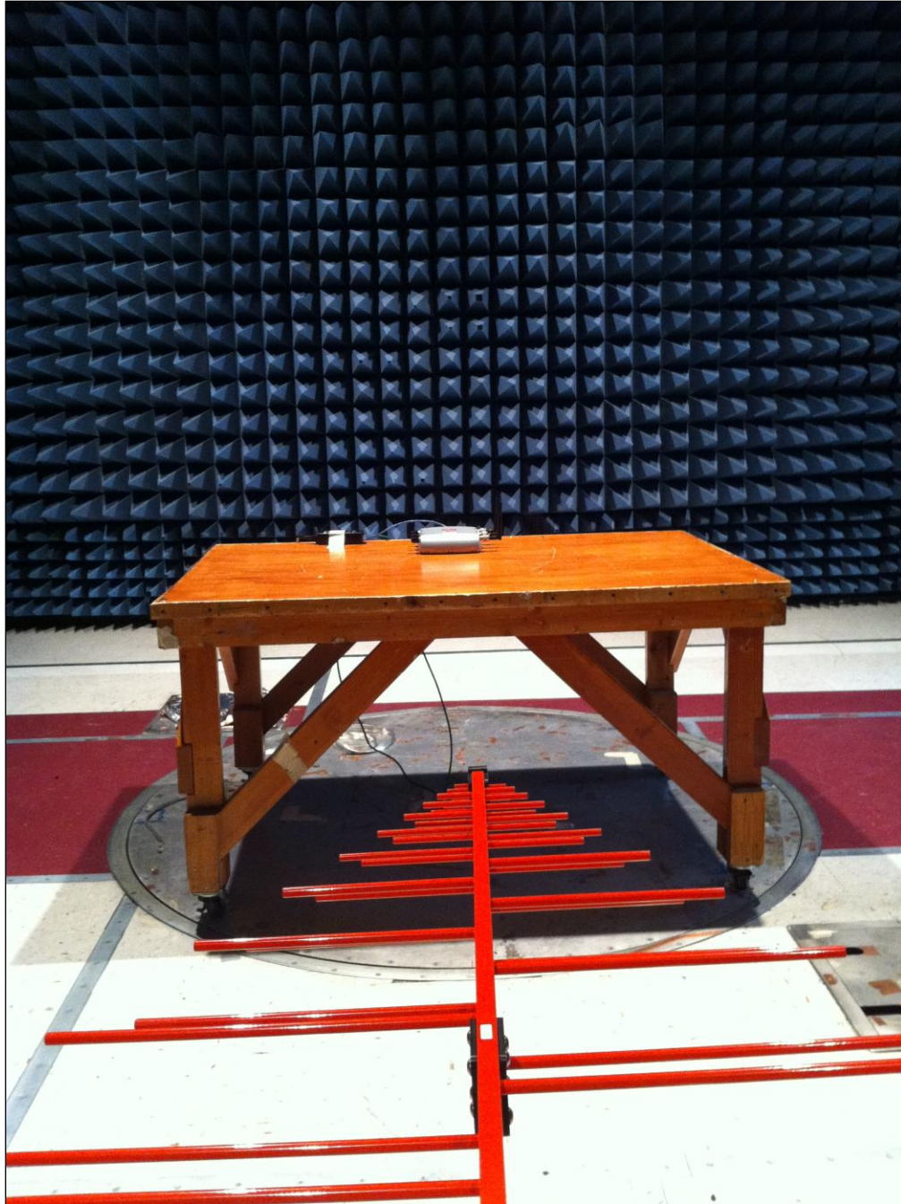
Photograph 7. Radiated Spurs, Test Setup, 5 dBi Omni, 30 MHz – 1 GHz
