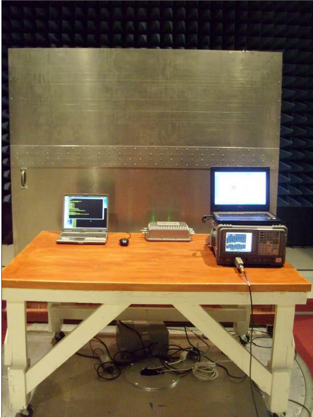
Photograph 6. Conducted Emissions, 15.207(a), Test Setup
