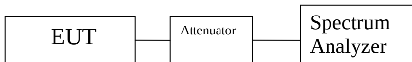
Figure 4. Power Output Test Setup
