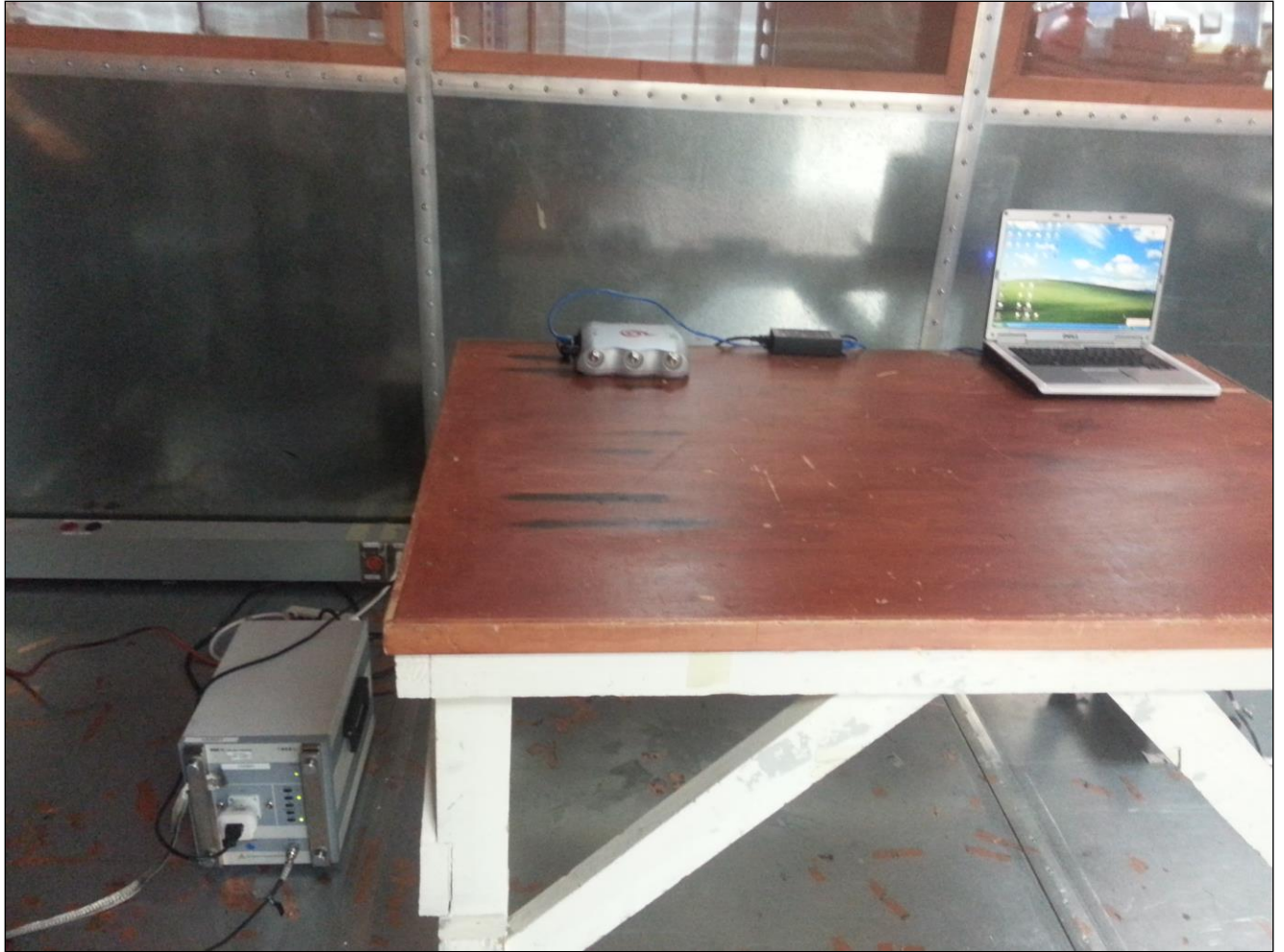
Photograph 6. Conducted Emissions, 15.207(a), Test Setup
