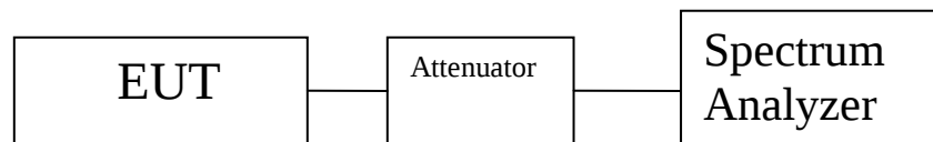
Figure 5. Block Diagram, Conducted Spurious Emissions Test Setup
