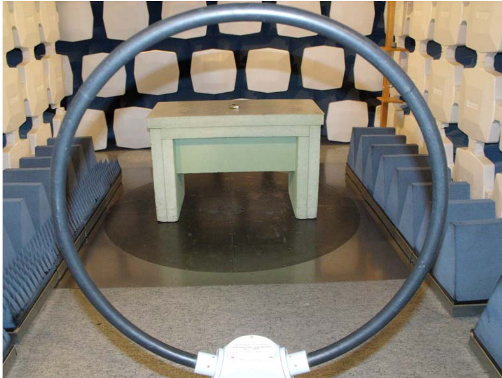
Figure 1: Radiated emission test – under 30 MHz
