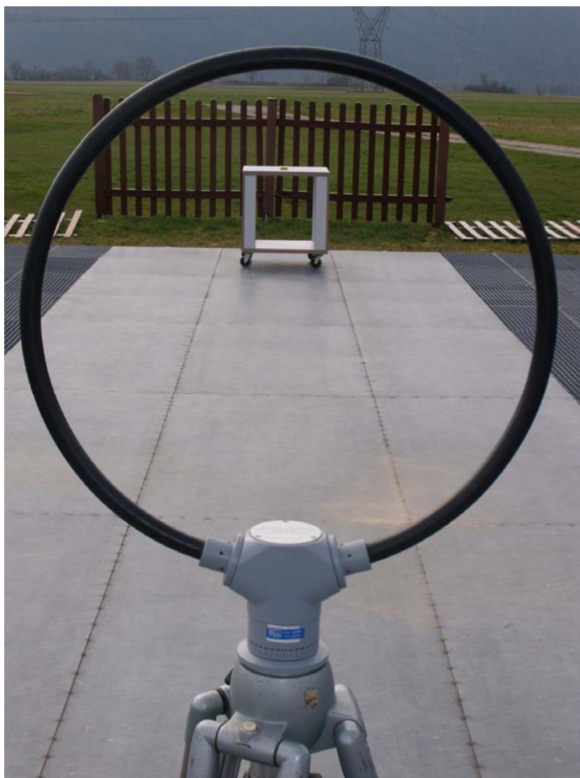
Figure 3: Radiated emission test – under 30 MHz on OATS
