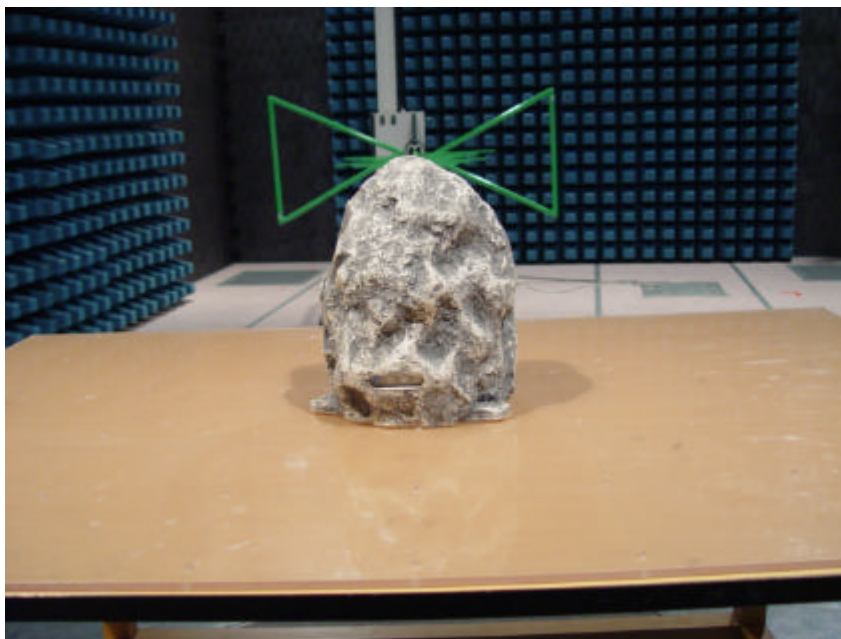
Photograph 2: Set-up for Radiation Measurement Below 1GHz
