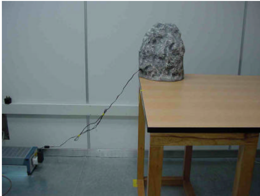
Photograph 1: Set-up for Conducted Emission on AC Mains
