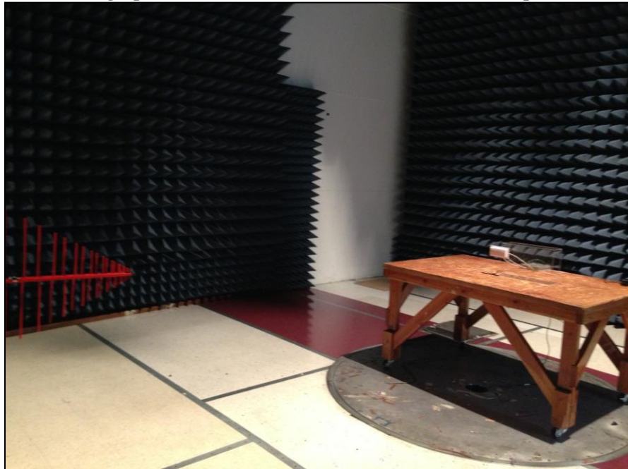
Photograph 10. Radiated Spurious Emissions, Test Setup, 30 MHz – 1 GHz, Ceiling Antenna
