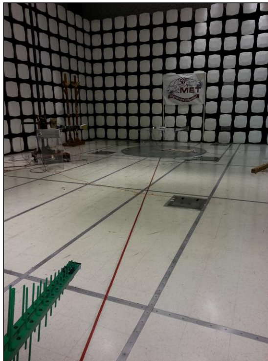
Photograph 6. Radiated Emission, Test Setup, PoE
