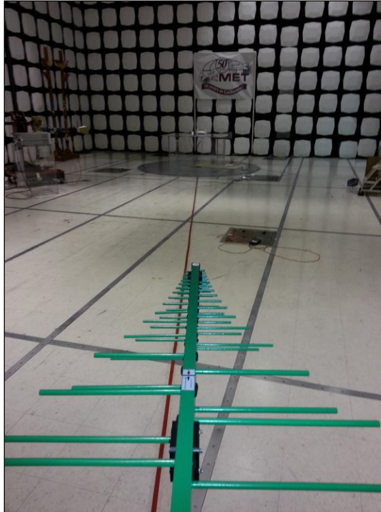
Photograph 5. Radiated Emission, Test Setup, AC-DC Power Supply
