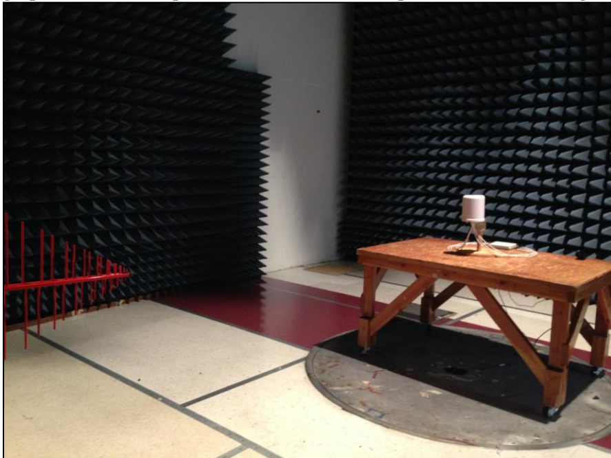
Photograph 12. Radiated Spurious Emissions, Test Setup, 30 MHz – 1 GHz, Omni
