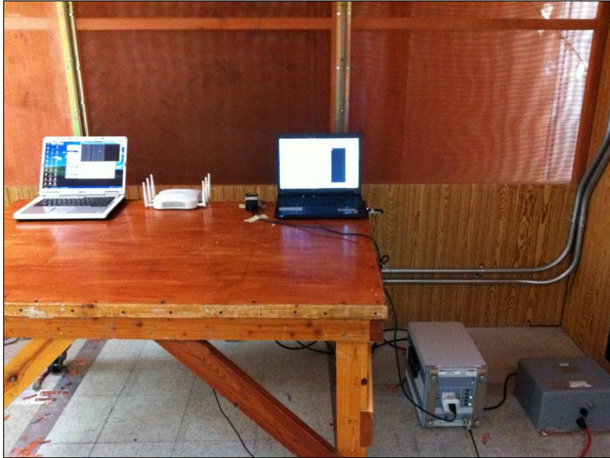
Photograph 3. Conducted Emissions, Test Setup, PoE, 1
