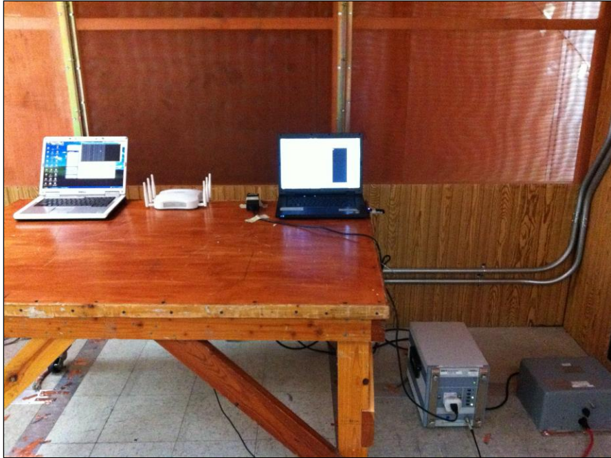
Photograph 9. Conducted Emissions, 15.207(a), Test Setup, PoE
