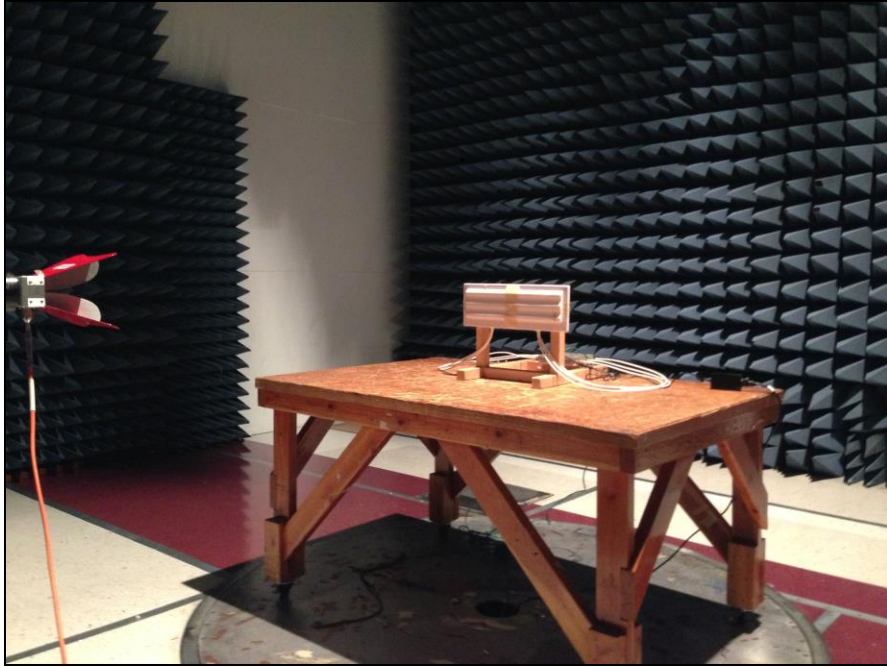
Photograph 15. Radiated Spurious Emissions, Test Setup, Above
