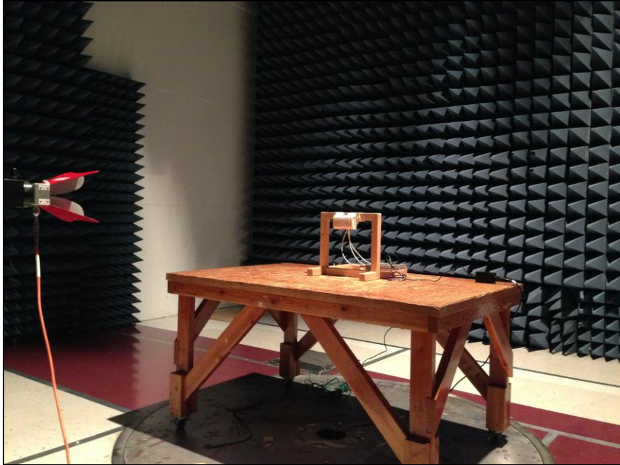
Photograph 11. Radiated Spurious Emissions, Test Setup, Above 1 GHz, Ceiling Antenna
