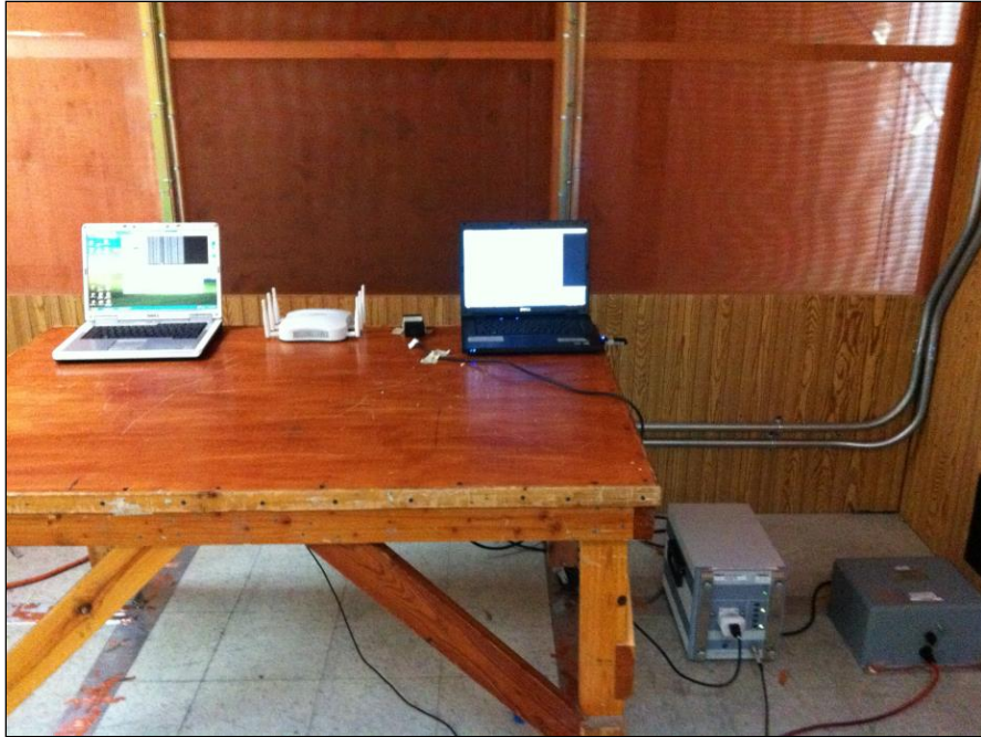
Photograph 1. Conducted Emissions, Test Setup, AC-DC Power Supply, 1
