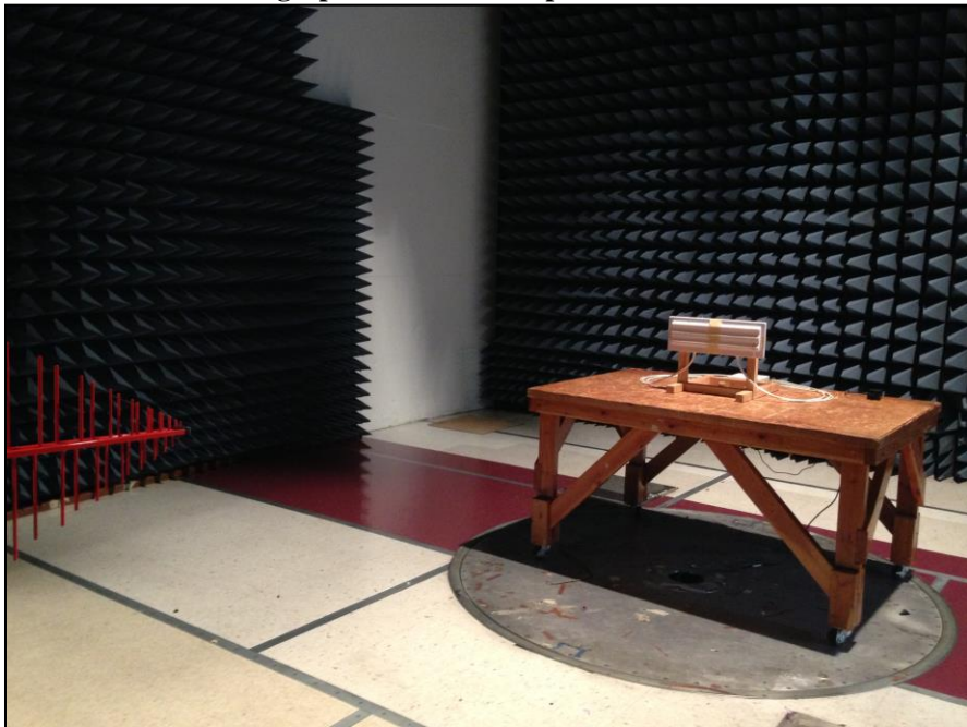
Photograph 14. Radiated Spurious Emissions, Test Setup, 30 MHz – 1 GHz, Patch Antenna
